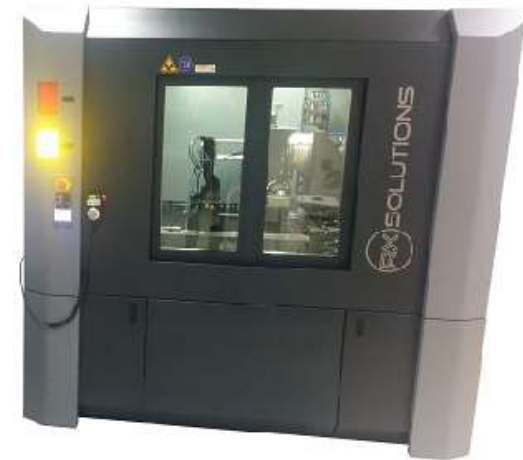
Nano computed tomography system 160 kV X-ray source Dual detector system with 1920 * 1536 pixel flat panel detector and 4032 * 2688 pixel CCD camera 50 nm min. voxel size
